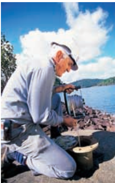
STEVE SCIBAN - KOOMBOOLOOMBA DAM MANAGER MEASURES WATER SEEPAGE LEVELS INSIDE THE KOOMBOOLOOMBA DAM SPILLWAY.
